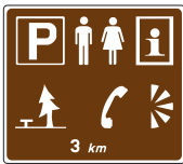
Advance sign for facilities in lay-by
