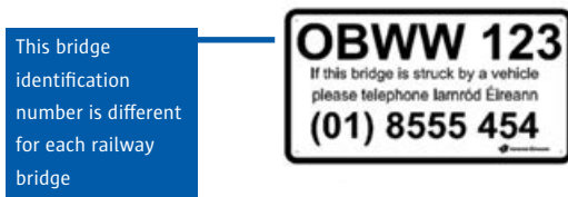
Example Railway Bridge Identification Plate
