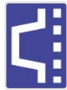
Emergency (Tunnel) Lay-by
